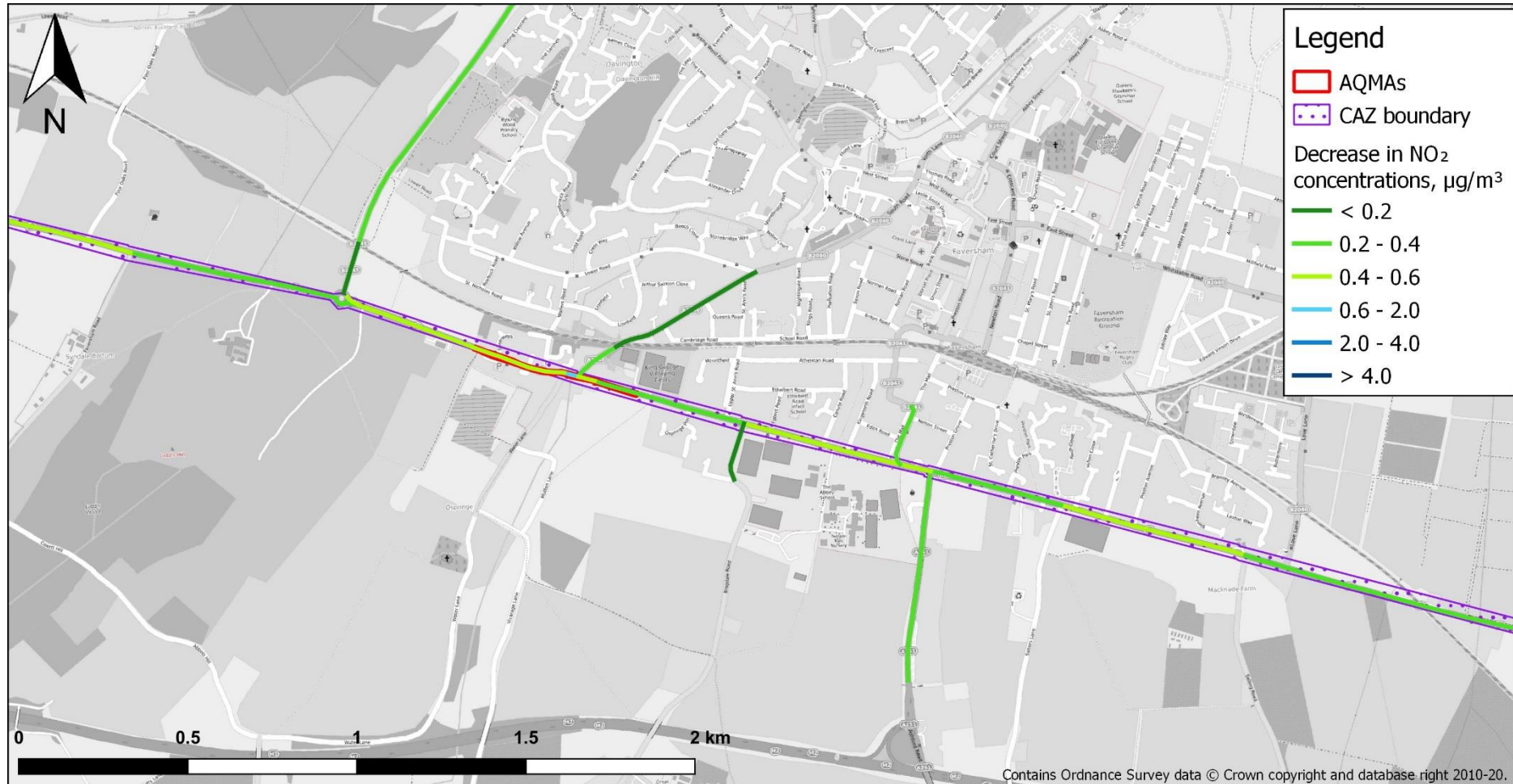
Figure 4-11 – The reduction in NO 2 concentrations around Faversham for the mode shift option
