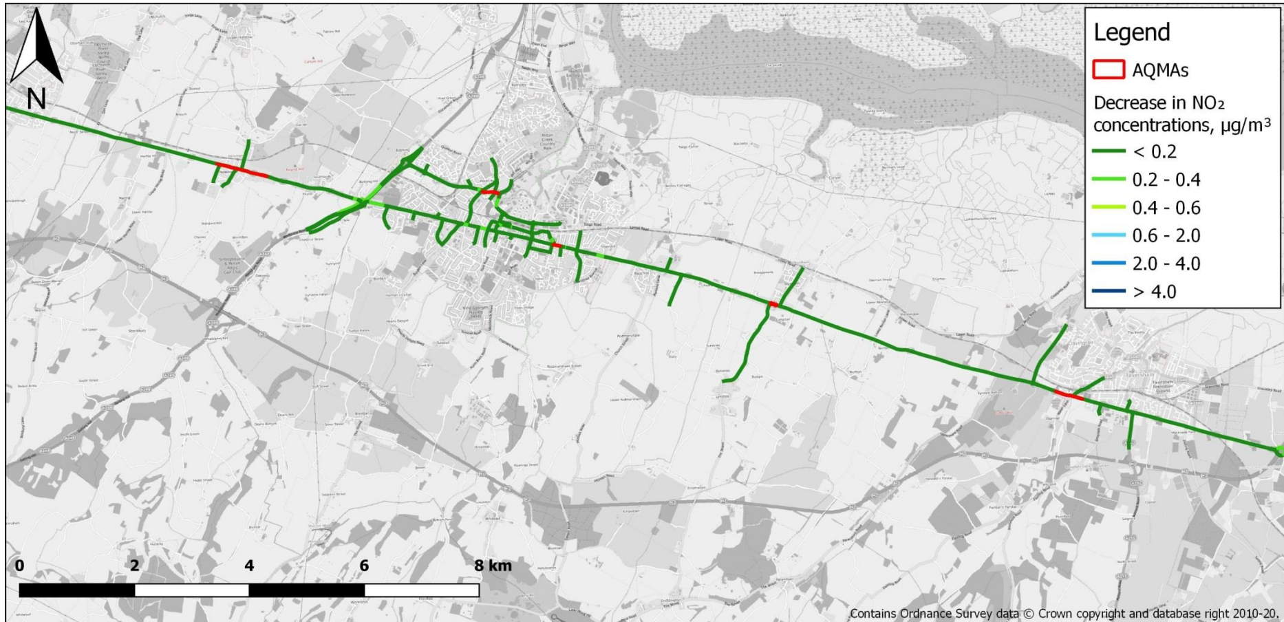
Figure 4-14 – The reduction in NO 2 concentrations along the A2 for the freight option
