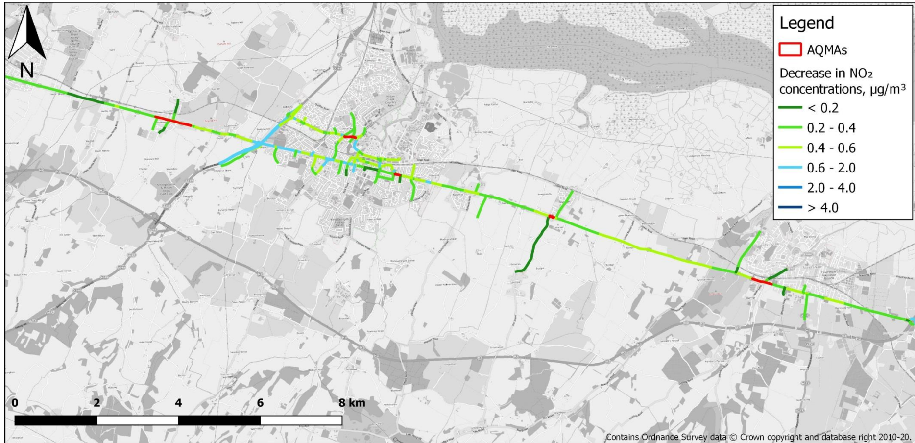
Figure 4-10 – The reduction in NO 2 concentrations along the A2 for the mode shift option
