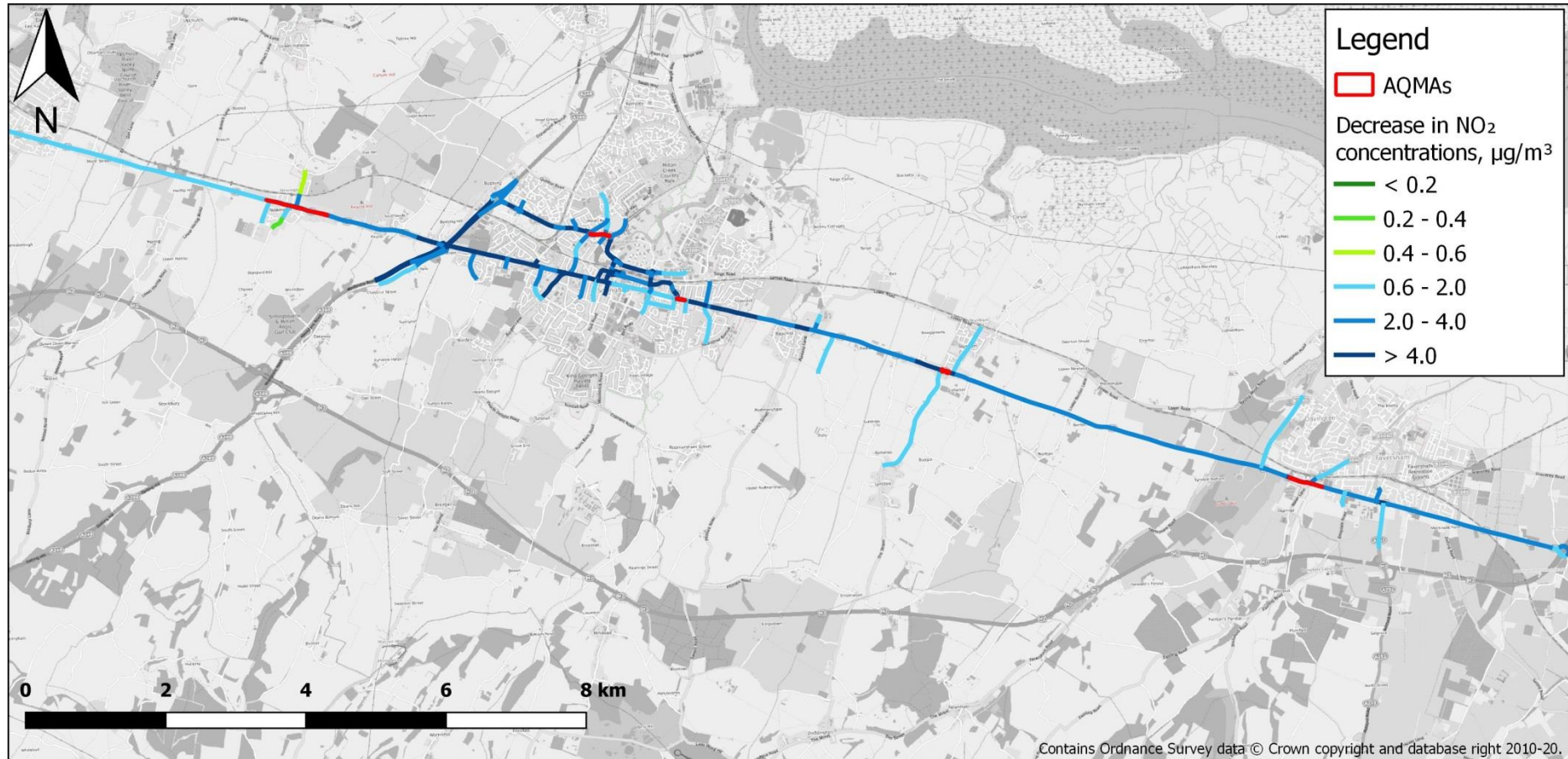
Figure 4-6 – The reduction in NO 2 concentrations along the A2 for the CAZ D option
