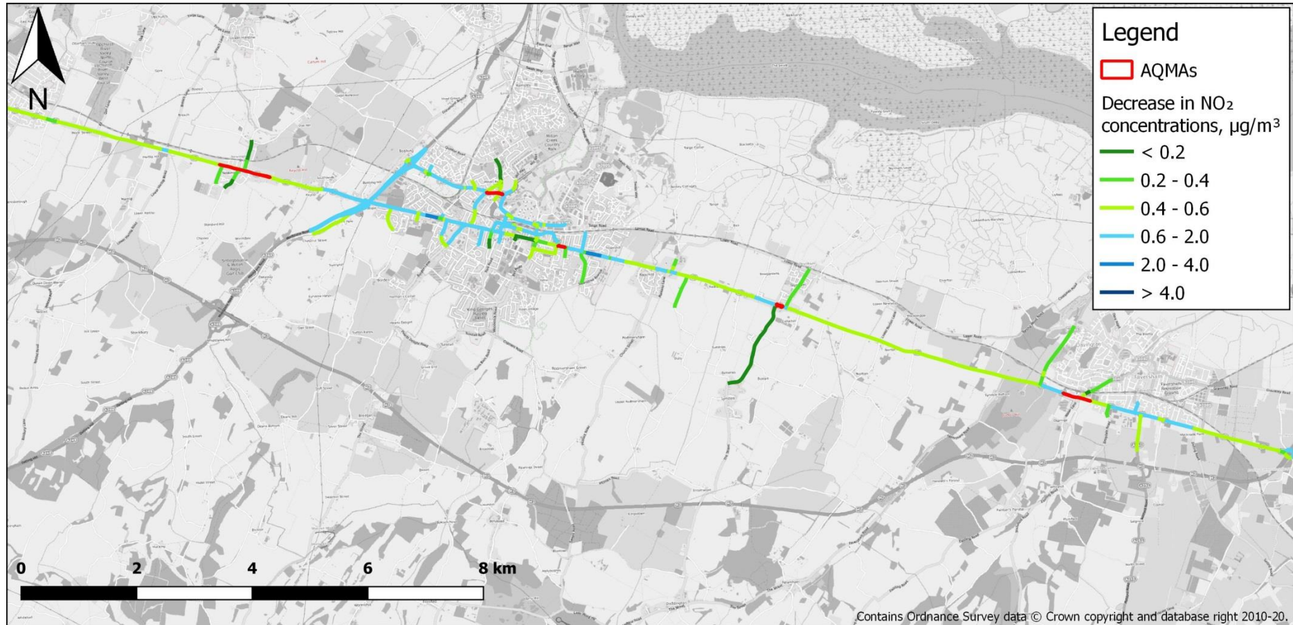
Figure 4-26 – The reduction in NO 2 concentrations along the A2 for the bundle combining all non-charging measures
